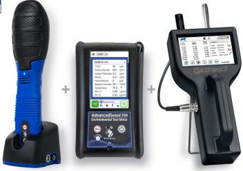
The PC-3500 can connect to GrayWolf's DirectSense XM probes and AdvancedSense XM meters (as well as other platforms) to combine 6-channel particle readings with up to dozens of other parameters into a single displayed and data-logged file.
